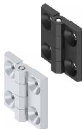
Screw-on hinge for countersunk screw M4; zinc die surface of choice; hinge pin stainless steel
